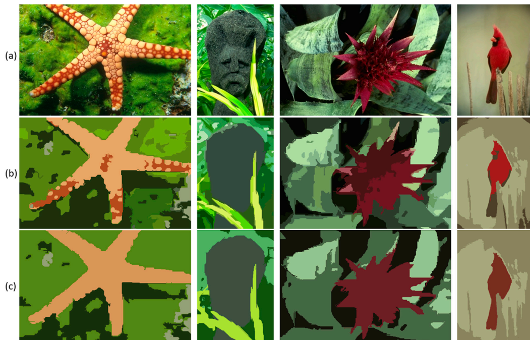
Figure 8. Comparison of segmentation results with and without K-means post-processing. From top to bottom: (a) Original images, (b) w/o K-means refinement, a lot of unwanted segment regions are formed (e.g., starfish has dark colored spots, flower is also segmented into two segments, and the same with the bird, as it has two different colored segments), (c) w K-means refinement step, one object is given only one label.
