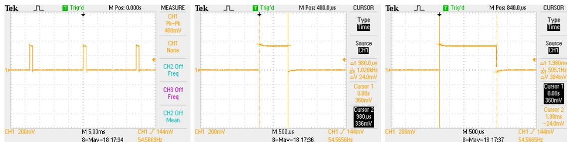
(a) Multiple pulses of constant time and frequency being received from the radio transmitter.
